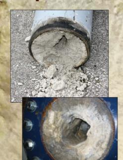
UNITED STRUVOUT™ prevents deposits of struvite from building up in lines within the wastewater treatment plant.
