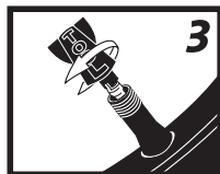
3. Replace Valve Core
